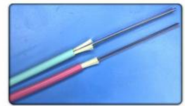
3.0mm MPO round fiber cable jacket stripping - Kevlar cutting at same by just one action.
