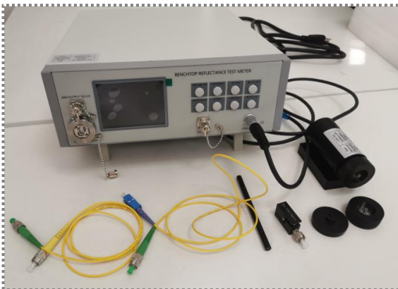
High power reception,for PLC WDM pigtail test
